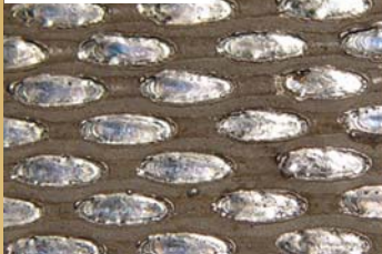
Coating designed to accommodate strain in 2-D.
